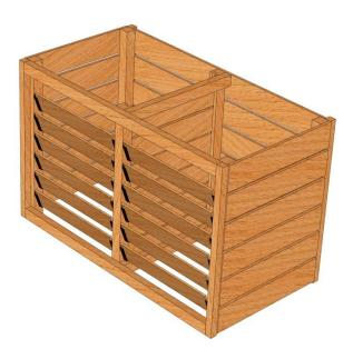
The composter consists of 2 separate bays with a removable dividing section. The divider and front slats can be removed for filling, emptying and transferring compost between the bays.
