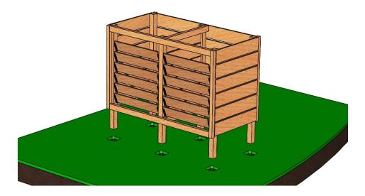
Before installation the area is marked out according to fig.15 to align with the corner posts, 900mm apart
