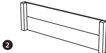
Fix a longer side board to the corner post as shown ensuring the end of the board sits neatly with the edge of post. (Fig 3)
